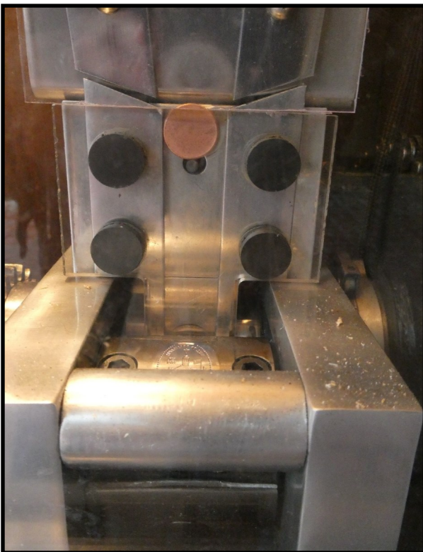
Rolling Machine in The Magic Kingdom near the Hall of Presidents with a zinc-copper blank in the slot waiting to drop onto the die for rolling. The raised rim is visible on the blank.
